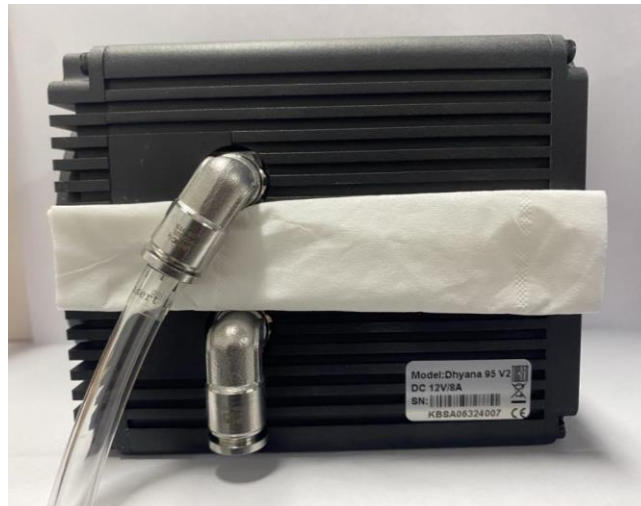
Figure 4-5 Removing the water-cooling pipes
