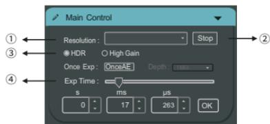
① Click the resolution drop-down box to select the working resolution of the camera.
